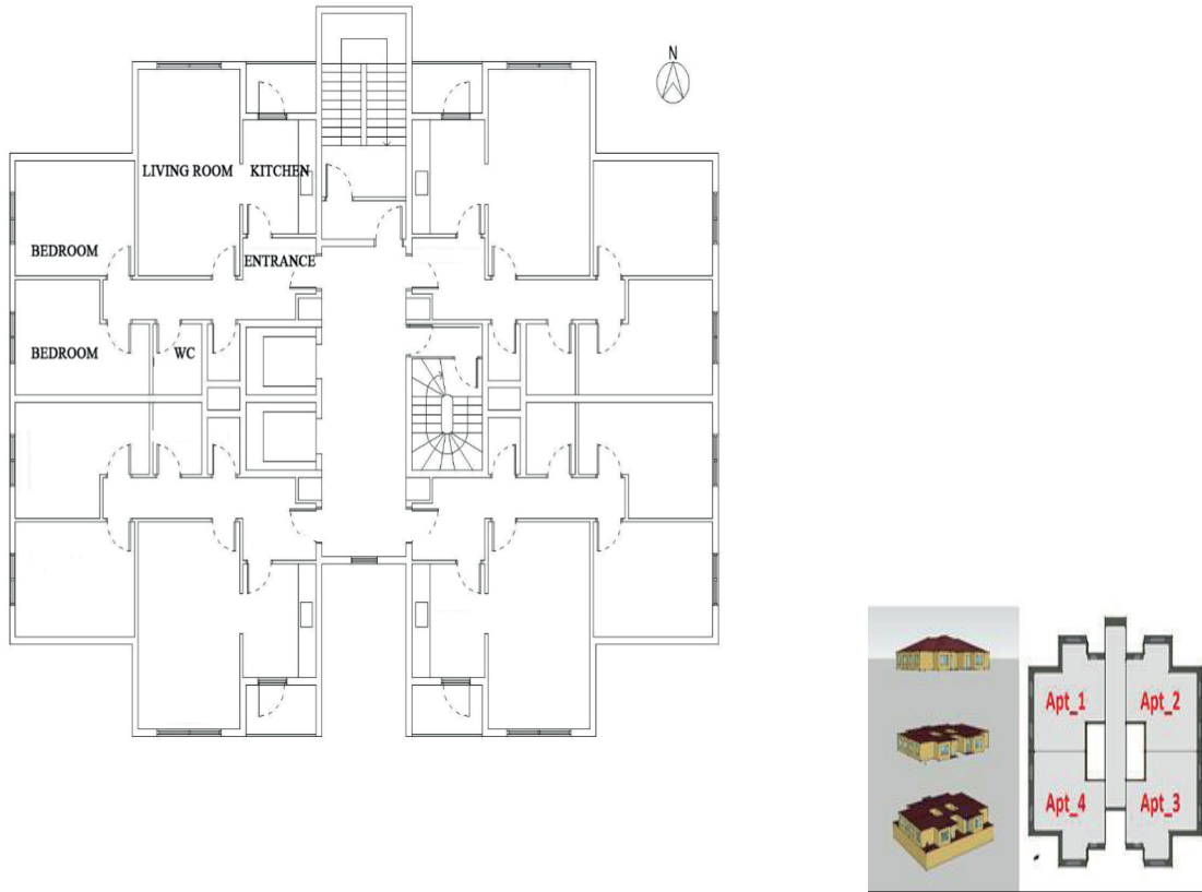
Figure 2. Typical Floor Plan of the Case Study Building (on the left) and the Thermal Zones of the Typical Floor (on the right)
